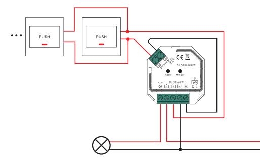
This phase dimmer adopts leading edge dimming (forward phase control) or trailing edge dimming (reverse phase control), two versions are available for choosing, default factory setting is trailing edge, leading edge version available upon request. Please make sure the connected loads support the control type you choose. Please refer to the user manual of the load or consult the supplier of the load.
